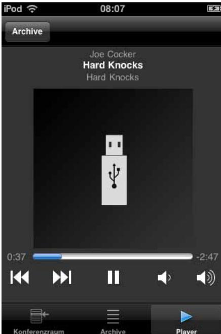
In the case of a USB stick, a cover is only displayed with MP3 tracks where the cover is embedded in the metadata. All other file formats just show a placeholder irrespective of whether a folder, cover or album file is available on the USB storage medium. Control is the same as with the Music server.
