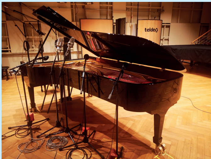
The mic set-up to capture the performance for SACD and Dolby Atmos included a series of Coles 4038 and Royer R121 ribbon mics as well as the classic Neumann M49 tube mics, amongst others.
