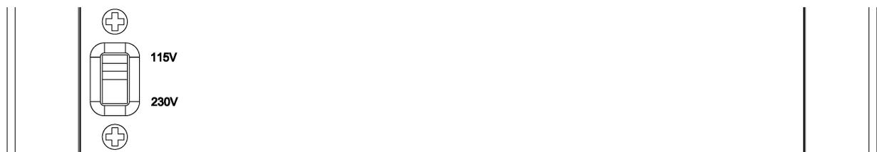
Make sure that the AC Voltage selector switch at the bottom of the unit is switched to the appropriate voltage for your country. All DAC-10H are shipped with the switch set to 230V AC in order to prevent accidental damage.
